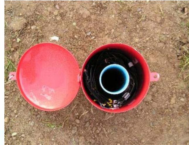
In spite of the presence of electrodes and cables, it is possible to acquire good-quality cross-hole GPR data using the same boreholes and a PulseEkko 100 system with 100 MHz antennas
