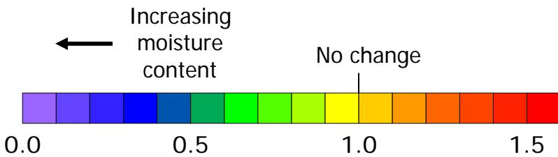
Ratio of resistivity at ground surface
